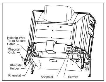
Figure 27 - Fan installation (Kit # 2767).
