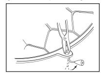
Figure 20 - Attach the griddle handle.
