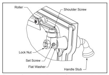
Figure 44 - Rotate pawl and/or remove flat washer to adjust latch.
