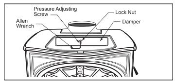
Figure 43 - Adjust the damper with the Allen wrench.
