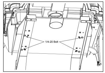
Figure 19 - Remove unit from shipping brackets.
