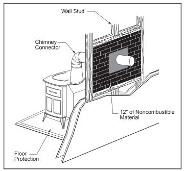
**Figure 10** - An approved wall pass-through for the United States. Three other methods are also approved by the NFPA:
