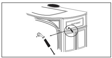
Figure 25 - Attach the thermostat handle.
