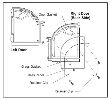
Figure 42 - An exploded view of the glass assembly.
