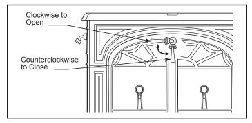
Figure 36 - To open the front doors, turn the handle clockwise.
