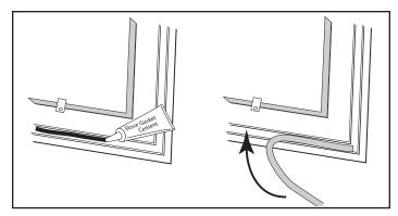
Figure 46 - Lay a bead of gasket cement then press gasket in place.
