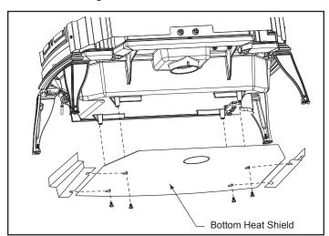
Figure 22 - Attach the bottom heat shield.
