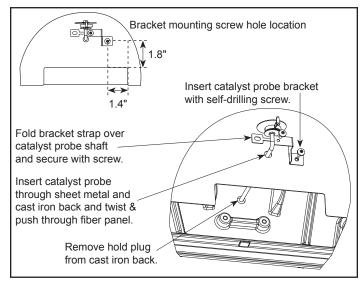
Figure 24 - Install the Catalyst Temperature Probe
