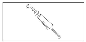
Figure 26 - Assemble the front door handle.
