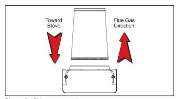
Figure 5 - Chimney connector.
