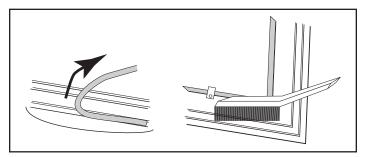
Figure 45 - Remove gasket then clean channel with wire brush.
