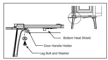
Figure 21 - Handle holder and heat shield positions.
