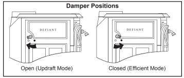
Figure 33 - The Defiant®'s damper operating positions.
