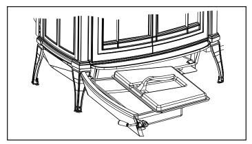
Figure 40 - Be sure the cover is securely attached before removing the ash pan.
