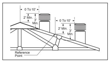
Figure 4 - The 2'-3'10' Chimney Rule.
