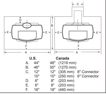
Figure 12 - Required floor protection dimensions.
