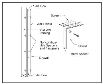
Figure 13 - Approved wall shield construction.
