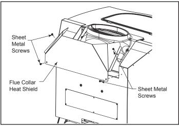
Figure 23 - Install flue collar heat shield.
