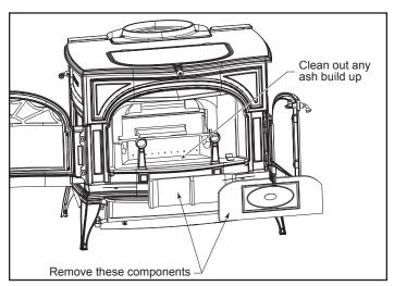
Figure 47 - Inspect and clean out ash accumulation behind the combustion system.
